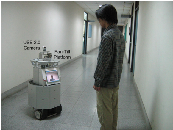
Fig. 10. Experimental mobile robot interacts with a user using a real-time face tracking algorithm and the proposed robust visual tracking control system.
