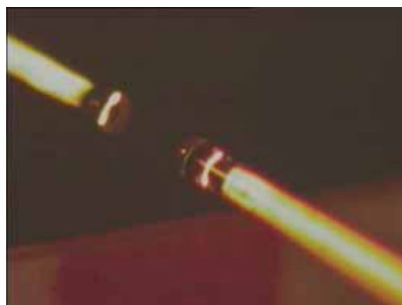
Fig. 4.12 The condition of fiberlens focusing laser on the sample.
