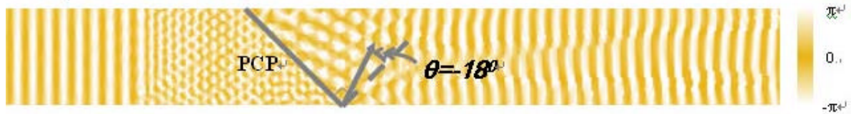
Fig. 16 This shows the refractive angle is -18^{\circ} at 16GHz
