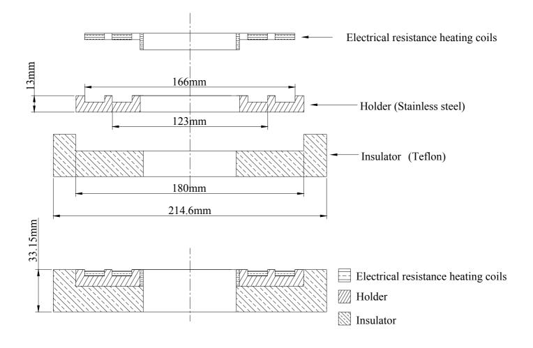
Fig. 2.3 The heater consists of three parts: resistance heating element, holder and insulator.
