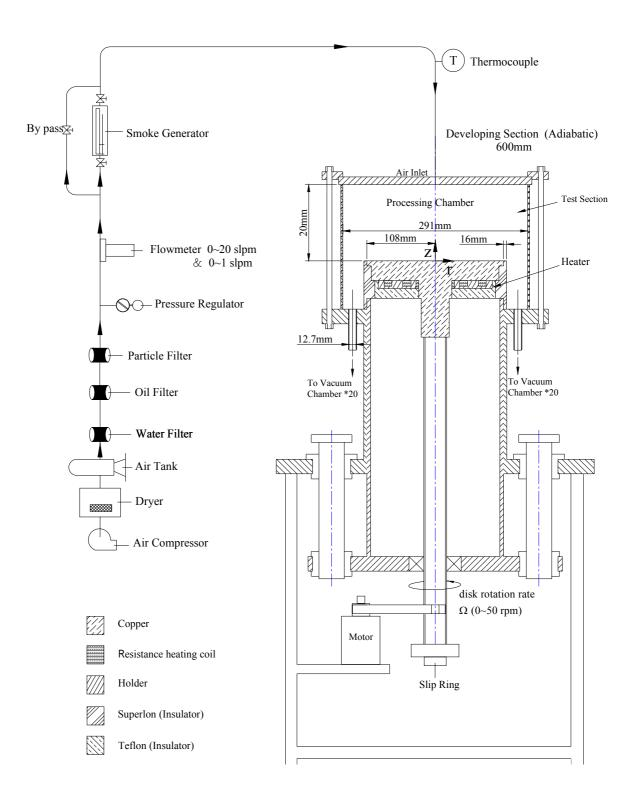
Fig. 2.1 Schematic diagram of the experimental apparatus.
