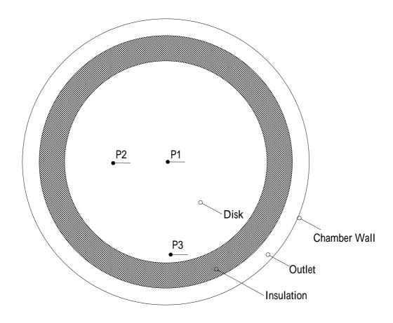
Fig. 2.4 The locations of the detection points on the upper copper plate.
