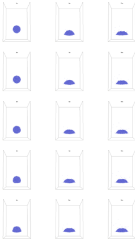
Figure 3.51 The evolution of the droplet impinging on the liquid film with the velocity 500m/s,
