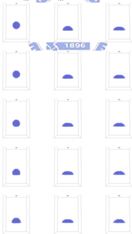
Figure 3.78 The evolution of the droplet impinging on the liquid film with the velocity 500m/s,
