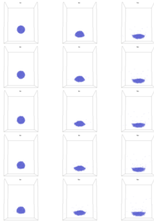
Figure 3.33 The evolution of the droplet impinging on the liquid film with the velocity 500m/s,
