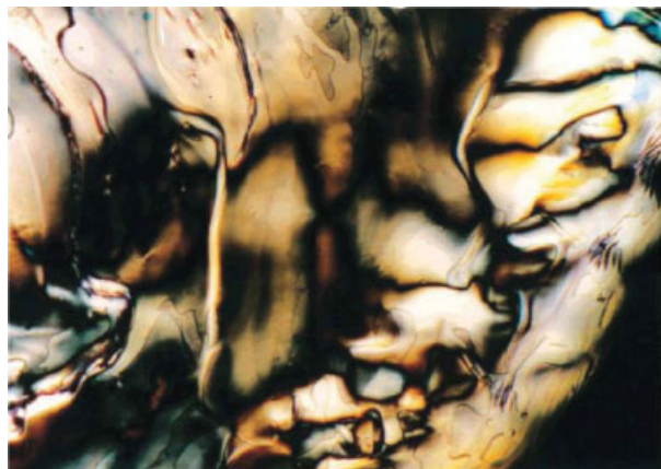
Figure 12. Optical texture of polymer P12 at 175 °C.
