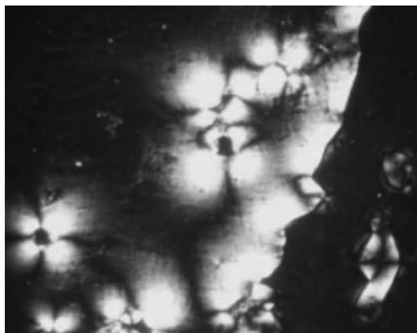
Figure 9. Optical texture of polymer P5 at 175 °C.
