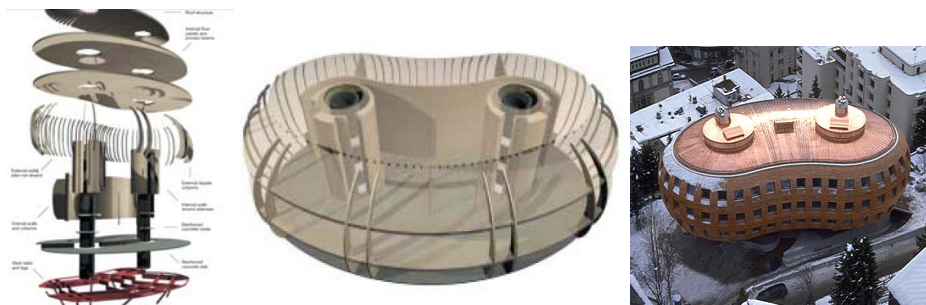
Figure 4-19. The Structural Elements
