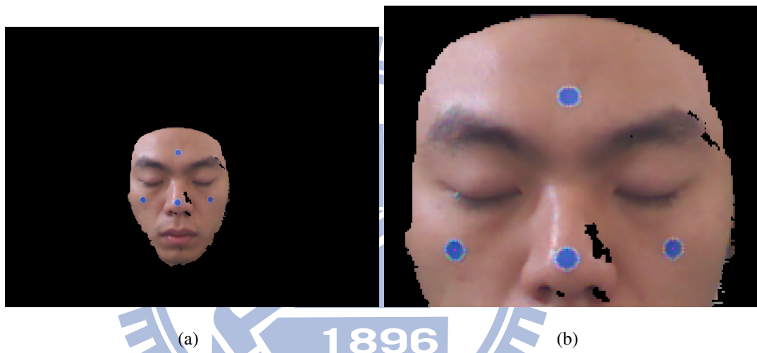
Figure 2.11: The result of estimation of centroid of markers. (a) The positions of markers on face. (b) After automatic estimation of centroid of markers, the centroids would found. The pink points are centroid of markers.
