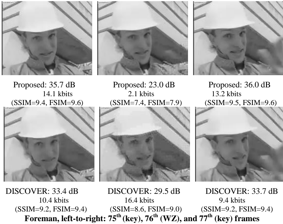
Fig. 18 Visual comparisons between the proposed codec (top row) and the DISCOVER codec (bottom row) at frame positions with highest PSNR variations. The bitrate of the proposed codec is 160.0 kbps, and the bitrate of DISCOVER is 161.6 kbps
