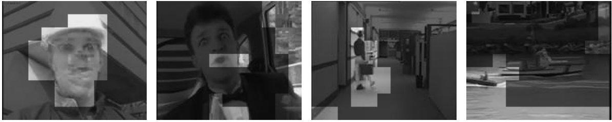
Fig. 14 Examples of ROI detection results. Macroblocks with normal gray levels are in \Omega_{ROI} .
