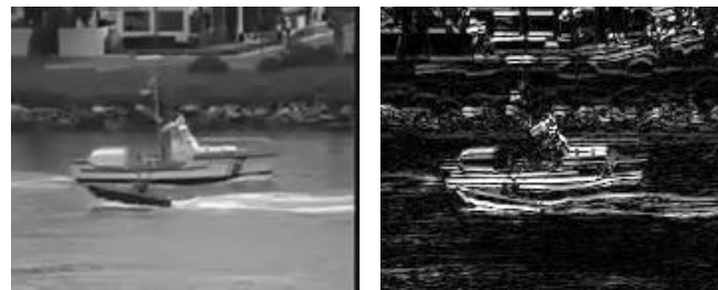
Fig. 21 The SI frame of the proposed codec (left) used in 0, and its error image (right). The SI frame of the DISCOVER codec is not available.
