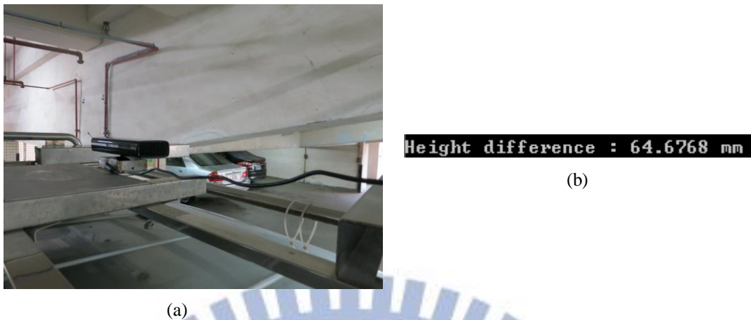
Figure 6.9 Results of monitoring height-restricting barriers. (a) Seen from the front top of the car. (b)
