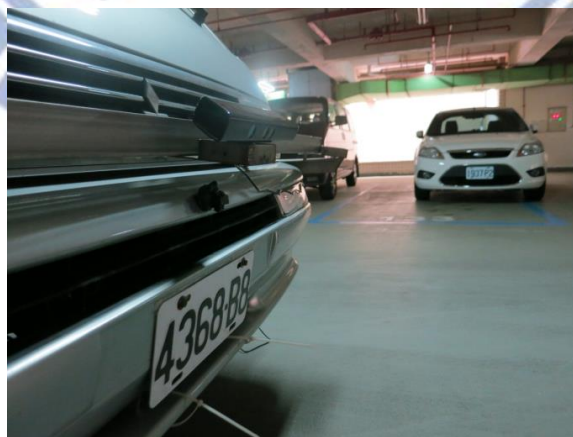
Figure 6.6 The KINECT device affixed in the front of the car which is tilted down thirty degrees.
