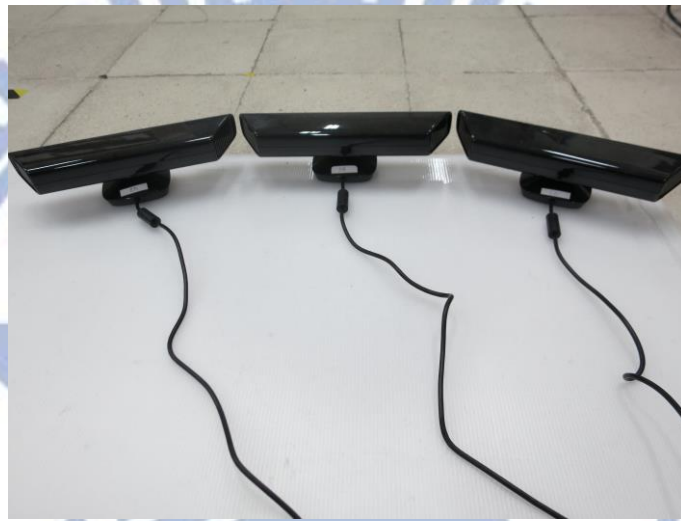
Figure 6.3 Three KINECT devices are affixed to the foam plank to simulate the video surveillance vehicle used in this study.
