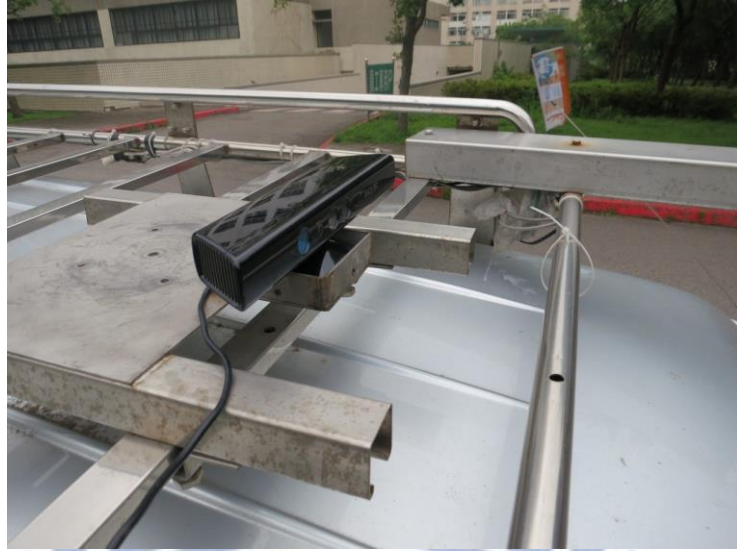
Figure 5.7 The KINECT device affixed on the front top of the car.
