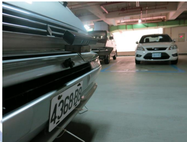
Figure 5.1 The KINECT device affixed in the front of the car and it is tilted down thirty degrees.
