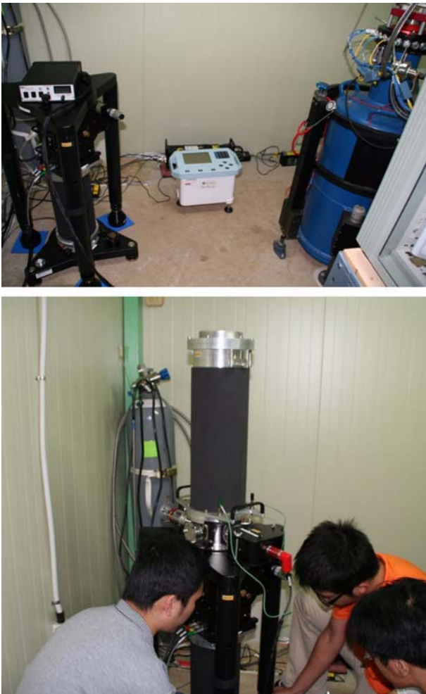
Fig. 2. Parallel gravimetric measurements at the MunGyung (Mungyeong) superconducting gravimeter observatory through absolute measurement by an FG5 gravimeter (black) and relative measurements from Graviton-EG (white with light blue top) and superconducting gravimeters (blue).
