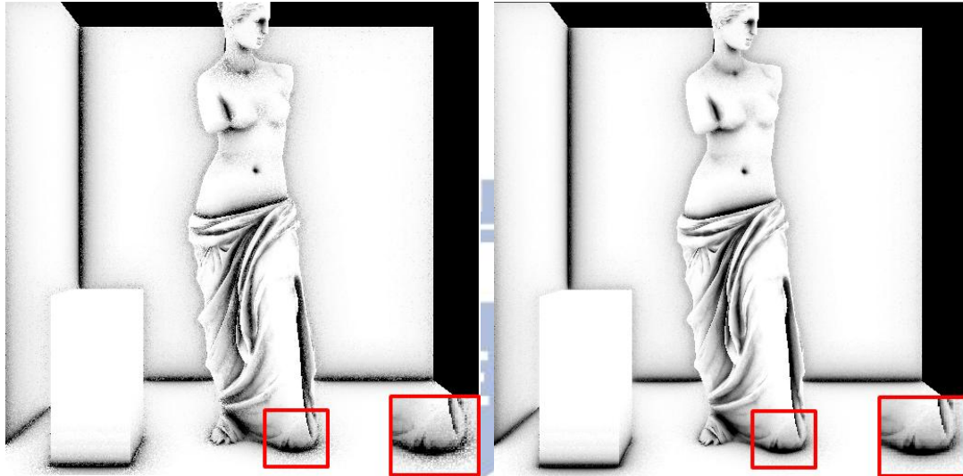
Figure 3.10: Both left and right SSAO use 32 samples per pixel. In the left image, SSAO without accumulating cached information has the noisy artifacts. In the right image, SSAO with accumulating cached information provides less noisy artifacts and maintains the details of the objects.
