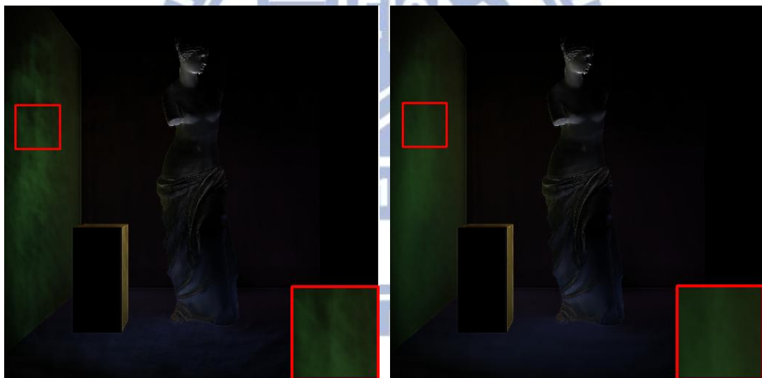
Figure 3.17: The comparison of indirect illumination with 512 VPLs. The banding artifacts are apparent without accumulating cached information (left). The result is smooth by accumulating cached information (right).
