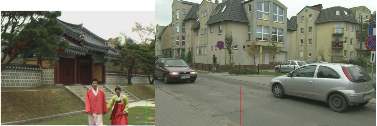
Figure 25: User marks lines on the floor (green line on the left and red line on the right) for calculating the 1-D floor model. The left and right images are Lovebird1 and Poznan_Street, respectively (MPEG test sequences).
