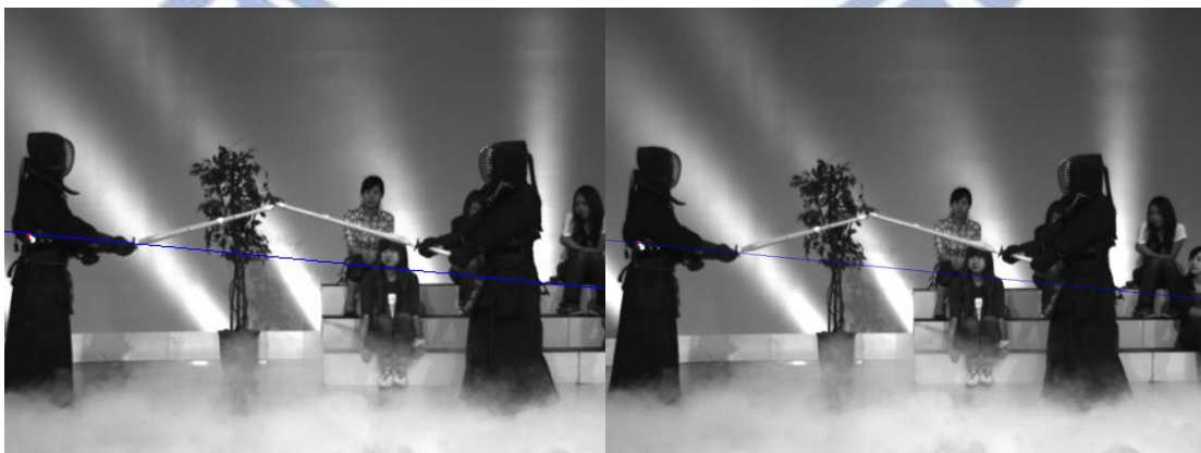
Figure 7: Epipolar lines for the two corresponding points
