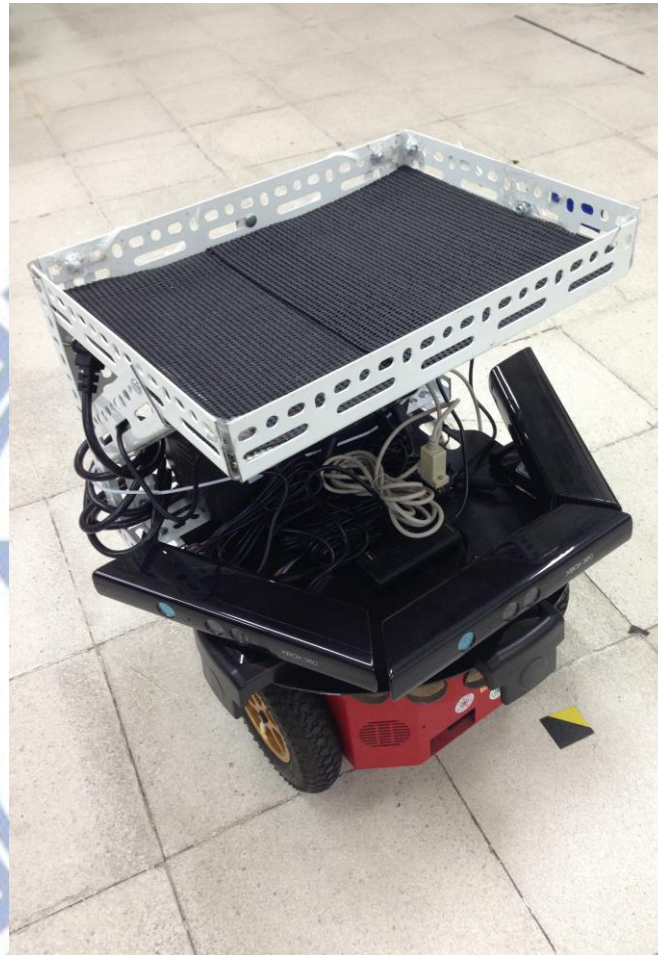
Figure 1.1 Image of proposed autonomous vehicle system with three KINECT devices.
