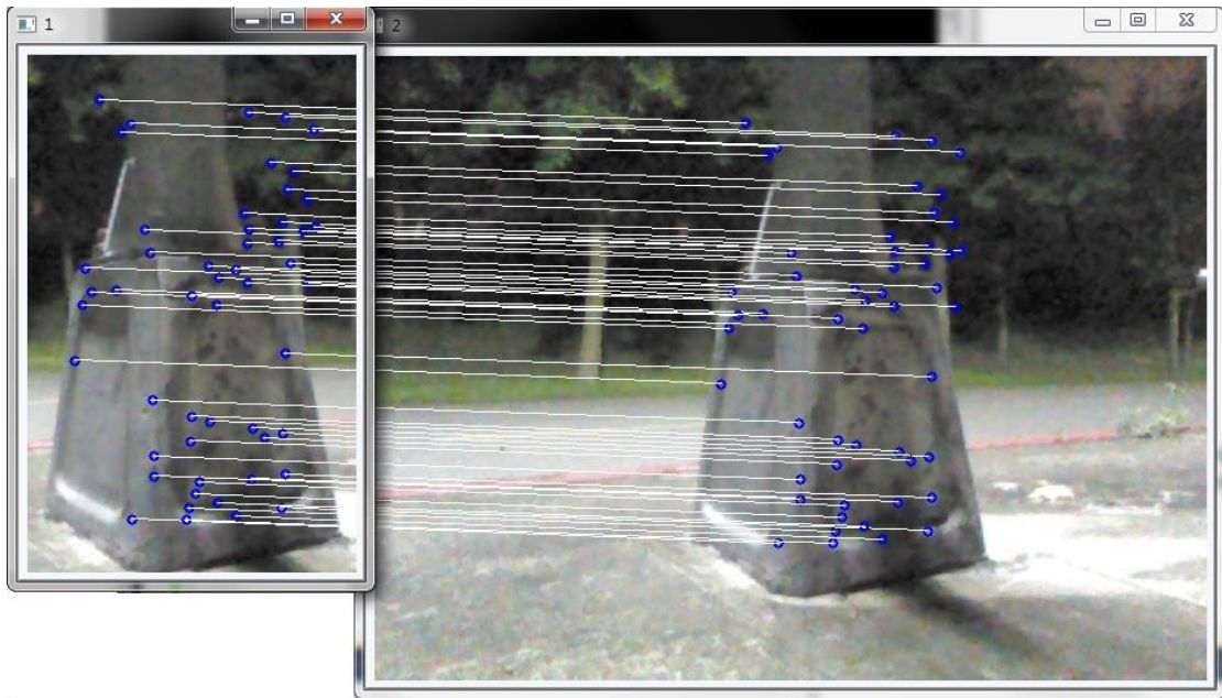
Figure 5.15 The matching result with the ROI image using the learned feature set.
