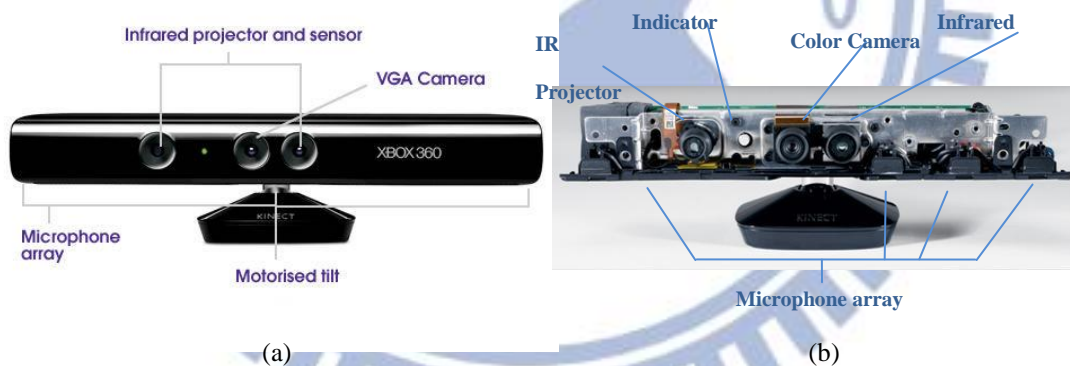
Figure 2.3 Hardware of the KINECT device. (a) Structure of external. (b) Structure of internal.
