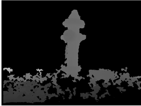
Figure 6.7 A depth image of a hydrant landmark with the ground information.
