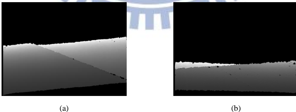
Figure 6.1 Two different perspective views of the curb on the sidewalk in the depth image acquired by a KINECT device. (a) A top-to-bottom view. (b) A farther view.
