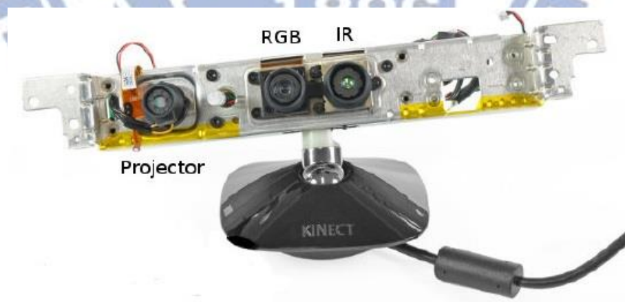
Figure 2.2 The KINECT device is composed of an Infra-red (IR) projector, an IR camera, and an RGB camera
