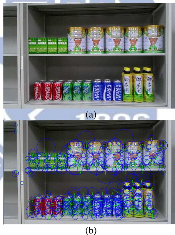
Figure 6.2 Feature extraction from client-camera images. (a) A client-camera image (b) Feature points of the client- camera image of (a).
