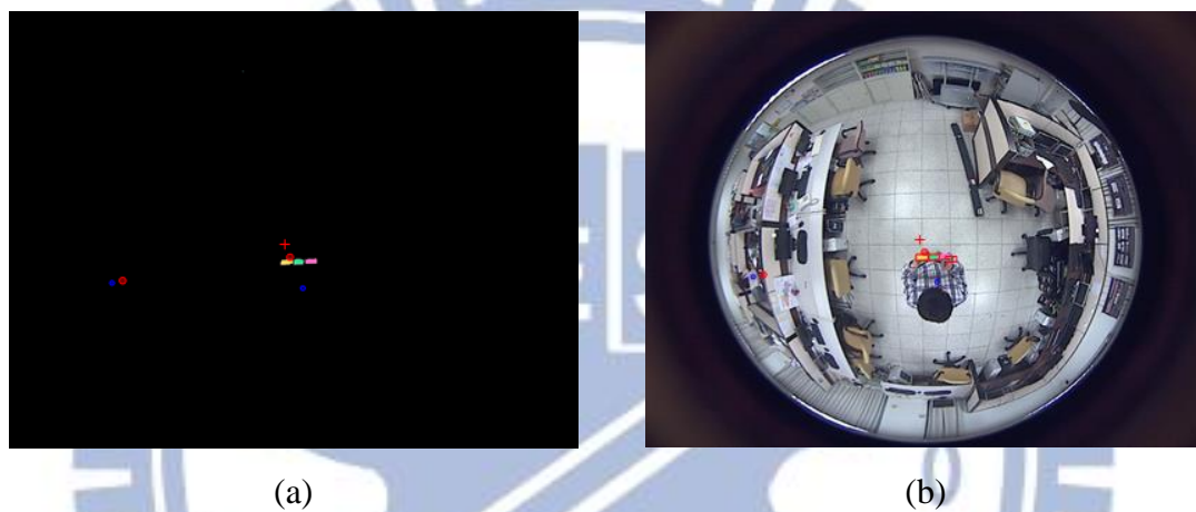
Figure 4.2 Detection of the color regions on the color edge mark on top of the mobile device. (a) The three color regions segmented from the omni-image. (b) The three bounding boxes (in red) detected in (a).
