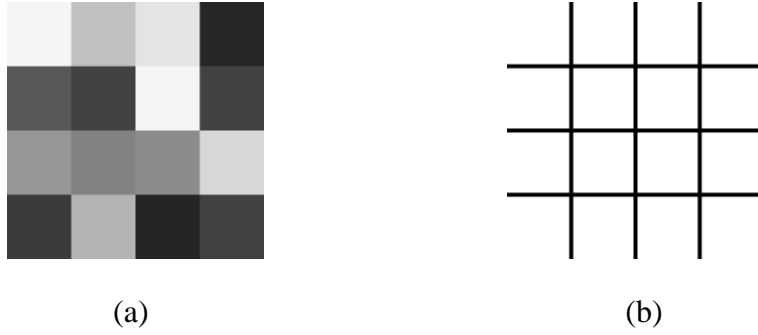
Fig. 1.3 The result of gray level edge detection. (a) The synthetic gray level image without noise; (b) The binary edge map obtained by Sobel operator [2] setting the threshold value T = 0.1 .
