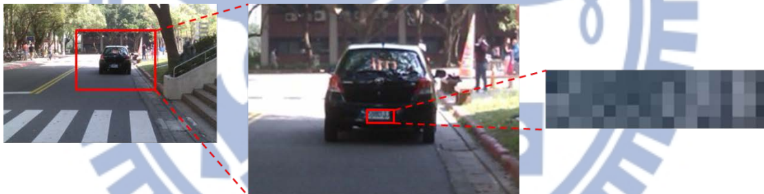
Fig. 1 An example of VLP region cropping from low resolution image.
