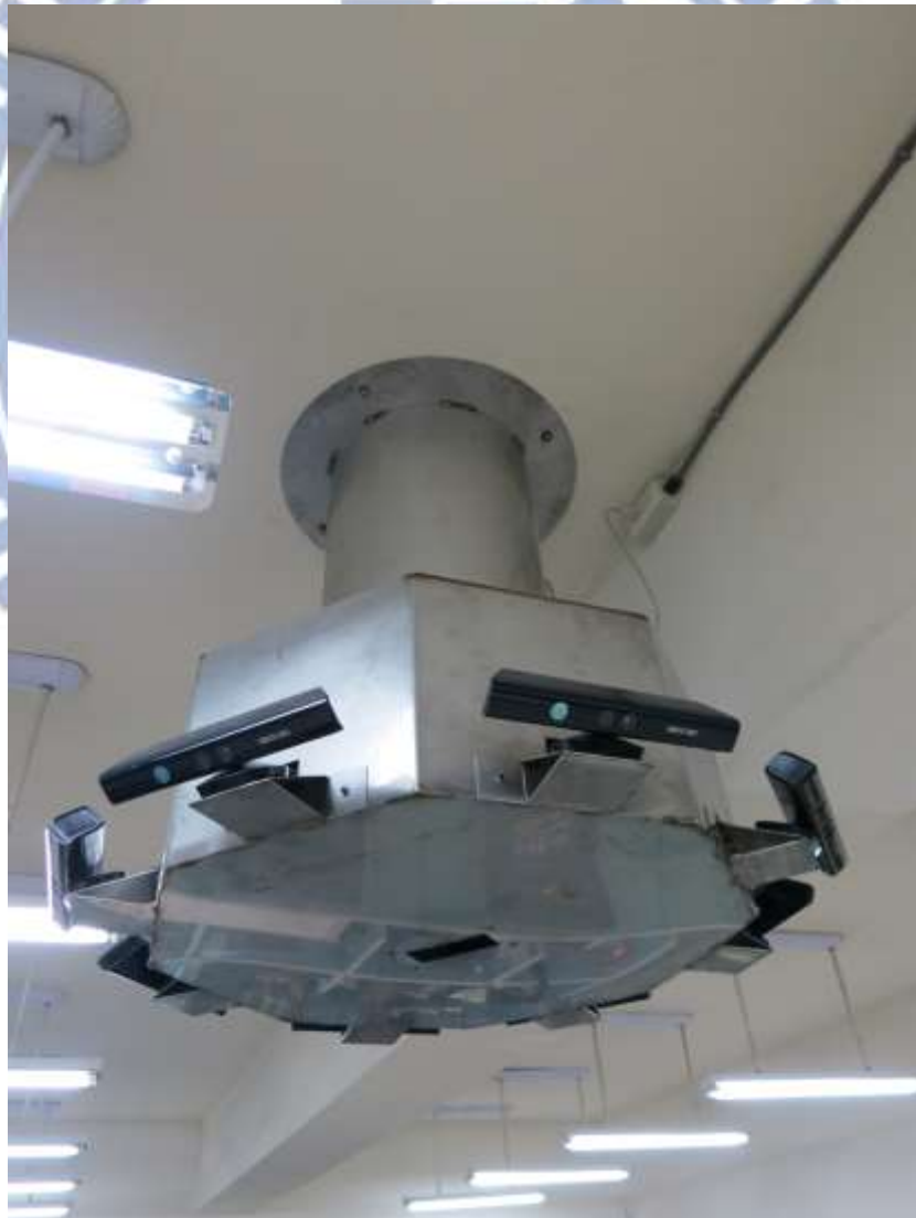
Figure 1.1 A picture of the proposed octagonal 9-KINECT imaging device.
