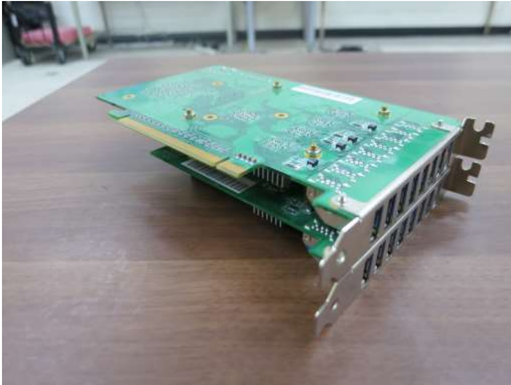
Figure 2.2 The Aguila SU16T Base is on the top of PCI Express x16 and the Aguila SU16T Expansion is at the bottom.
