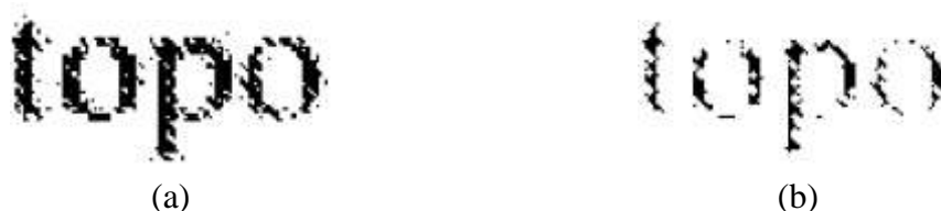
Figure 6.2 An example for erosion results. (a) The original image. (b) The image after erosion.
