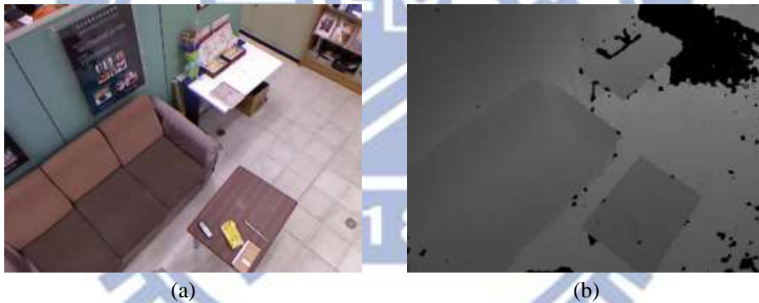
Figure 4.1 An example of a KINECT image pair. (a) The color image. (b) The depth image.
