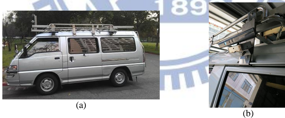
Fig. 3.5. Ferrous boxes for holding KINECT devices. (a) With a KINECT device. (b) Without a KINECT device.
