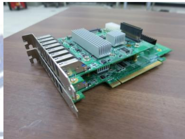
Fig. 2.2 The USB extension card (the upper is the expansion and the lower is the base)
