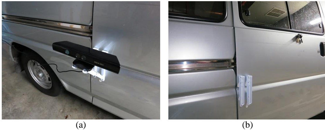
Fig. 3.4. A car-side iron stand for holding a KINECT device. (a) With a KINECT device. (b) Without a KINECT device.
