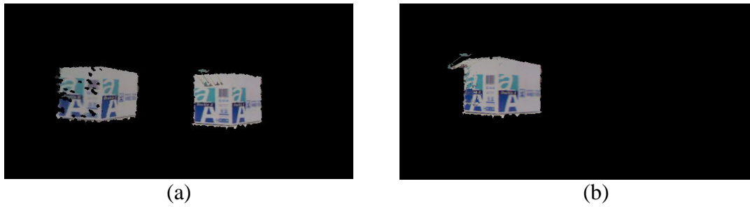
Fig. 7.2 Result of calibration. (a) Two 3D images seen before calibration. (b) A single 3D image seen after calibration
