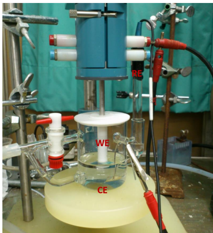
Figure 3.3 Three-electrode electrochemical system with a rotating disk electrode, where the WE is the working electrode, the CE is the counter electrode, and the RE is the reference electrode (Ag/AgCl).
