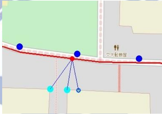
Figure 5.7 Vehicle localization by using multiple features. (a) The omni-image acquired from the camera. (b) A binary omni-image, in which the red lines indicate detected line features. (c) The map showing the position of vehicle, where the red point is the position of the vehicle and the blue points are the positions of the detected features.
