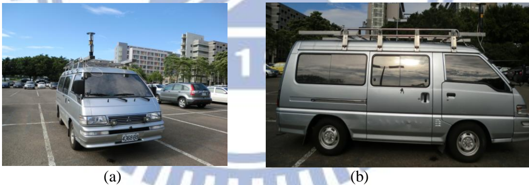
Figure 2.1 The video surveillance vehicle used in this study with an omni-camera affixed on the car roof. (a) A front view of the vehicle. (b) A side view of the vehicle.
