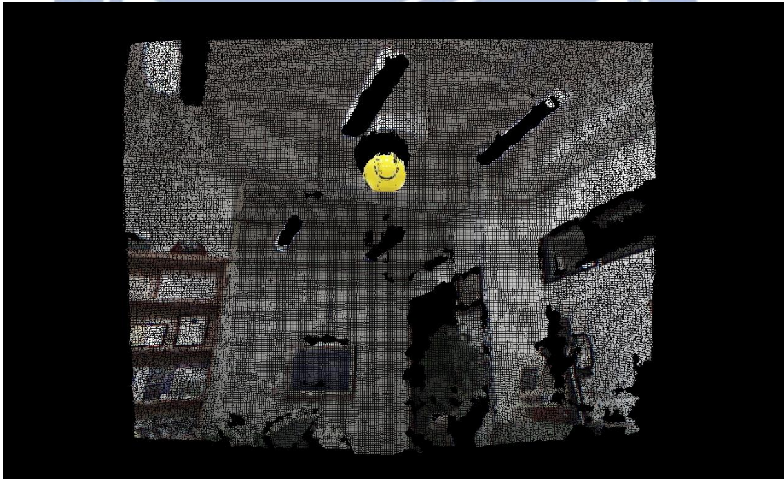
Figure 5.7 The watermarked 3D image in which the recovery data string is embedded by the difference expansion method.
