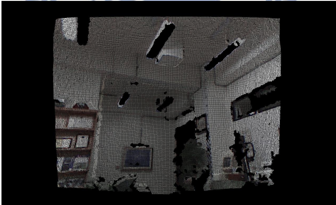
Figure 5.9 The result of combining the original depth and color image into a 3D image.
