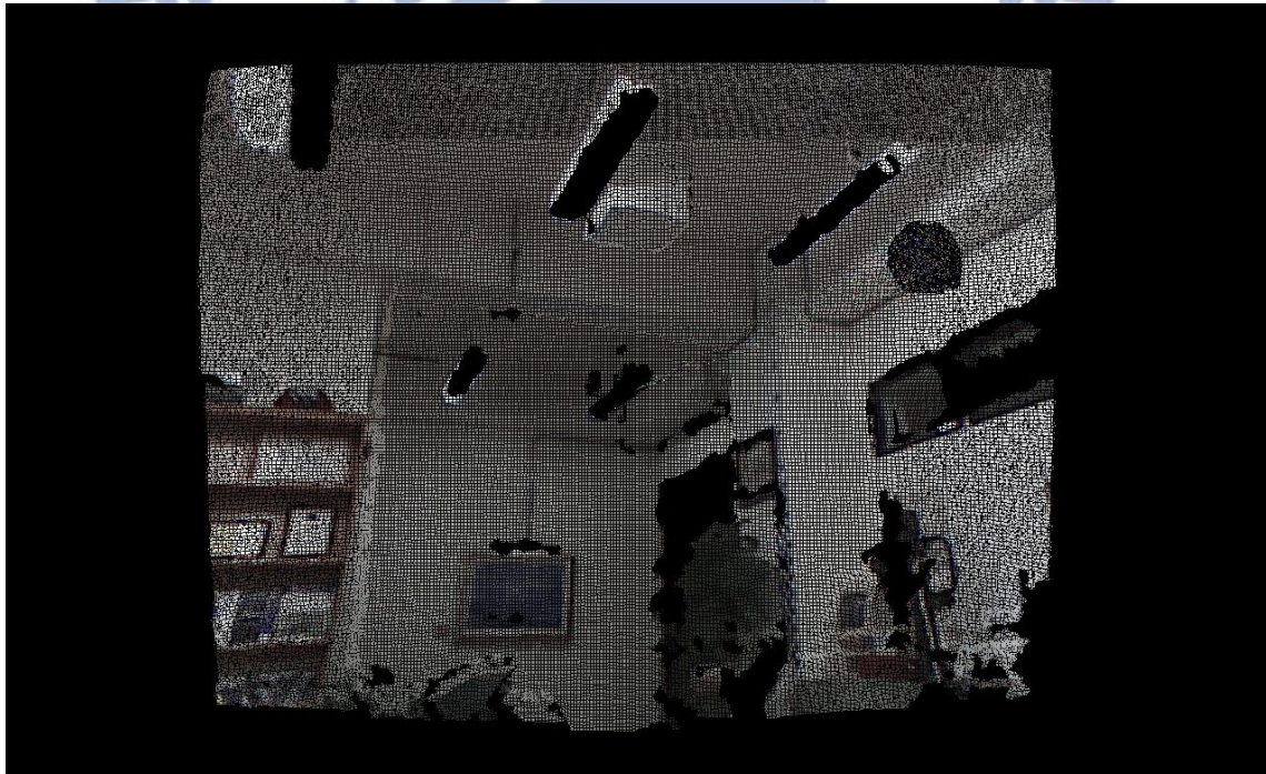
Figure 5.22 The result of eliminating the 3D watermark and recovering the covered region by using the wrong secret key to extract the hidden data.
