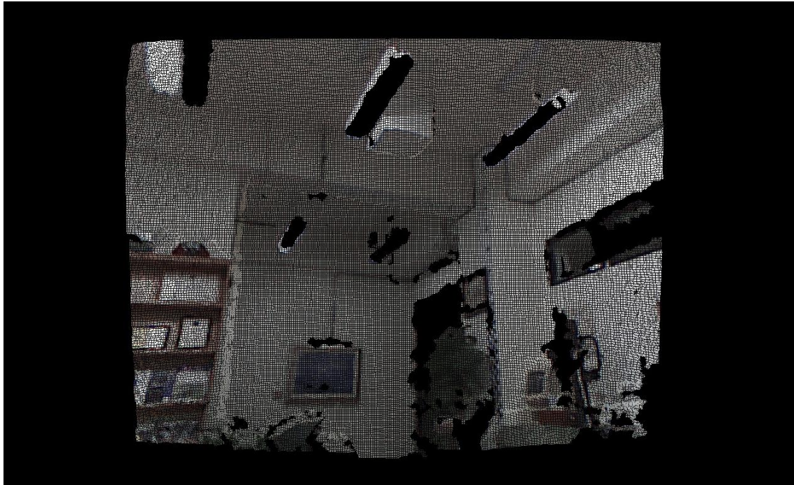
Figure 5.4 The result of combining the original depth and color image into a 3D image.
