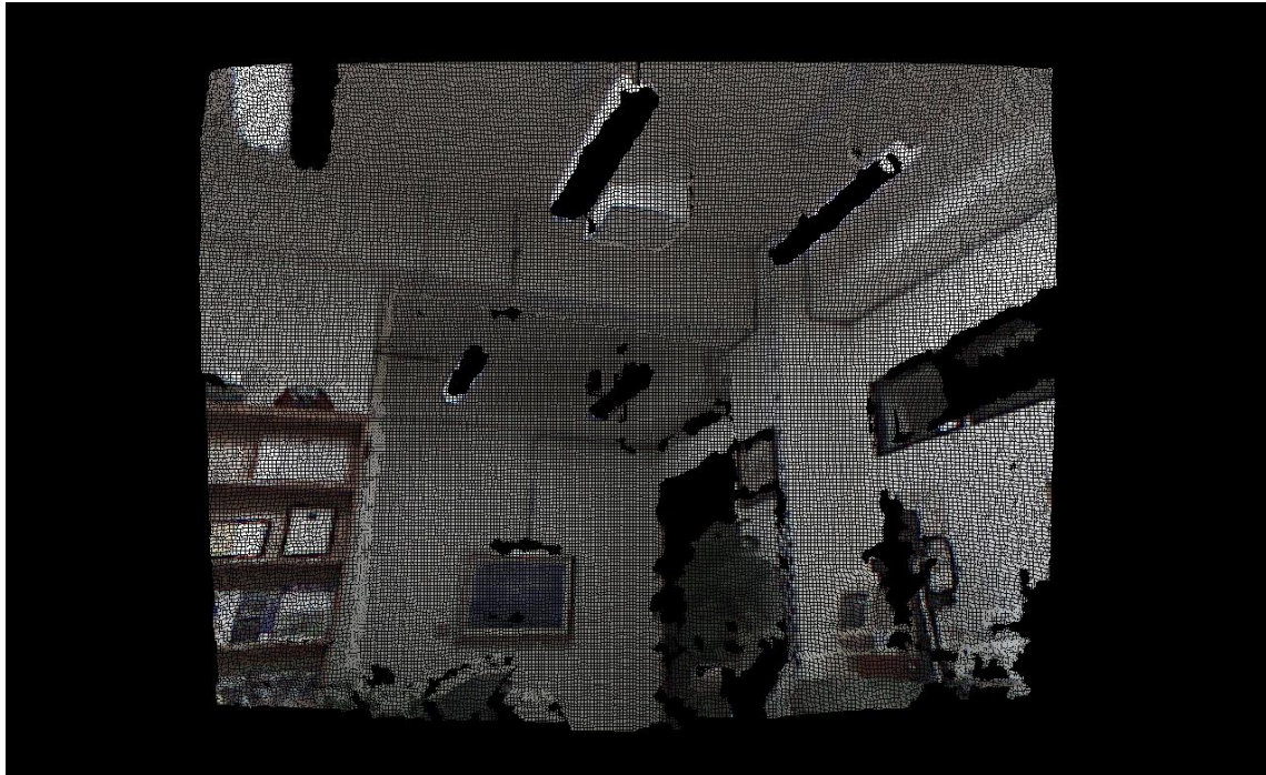
Figure 5.21 The result of eliminating the 3D watermark and recovering the covered region.
