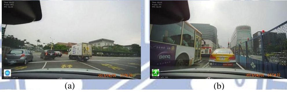
Figure 18. Conditions for the Ego-Motion Detector to behave incorrectly (a) Passing an open sky area (b) A high-height vehicle comes and stops nearby after cool-down is completed.
