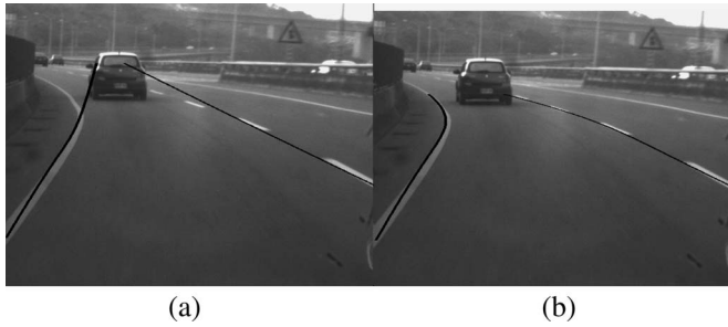
Fig. 23. Results of road scenes with a curve lane and occlusion. (a) Results of Jung and Kelber's approach [28]. (b) Results of the proposed approach.
