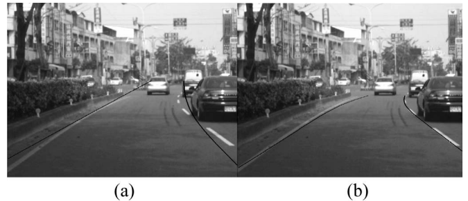
Fig. 22. Results of the road scene that the lane markings are occluded with shadows, signs of braking. (a) Results of Jung and Kelber's approach [28]. (b) Results of the proposed approach.
