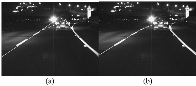
Fig. 25. Results of the nighttime road scene. (a) Results of Jung and Kelber's approach [28]. (b) Results of the proposed approach.
