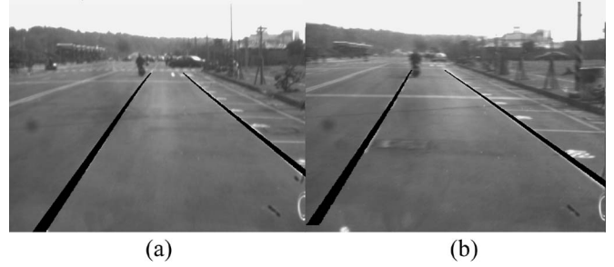
Fig. 21. Detection result of a motorcycle inside and outside the lane. (a) Inside. (b) Outside.
