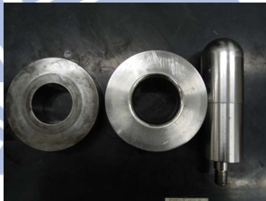
Figure C.6: The mold and punch of a universal deep drawing testing machine.
