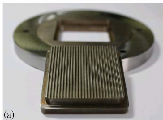
Figure 3.10: (a) A mold for hydroforming, and (b) geometries of micro-flow channels on the mold.
