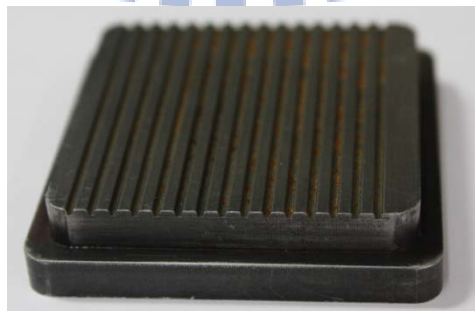
Figure 4.10: A mold of the verification experiment.
