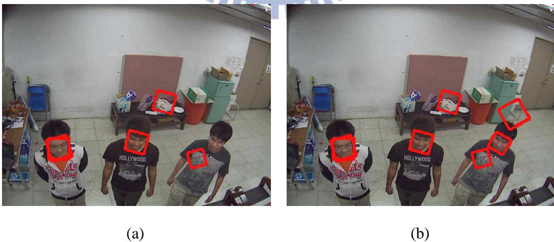
Figure 4.10: Combine the detection results of Figure 4.9 into one image. (a) Combine Figure 4.9(a)-(c) and 2 TP/FP in the image. (b) Combine Figure 4.9(a)-(e) and 3 TP/FP in the image.
