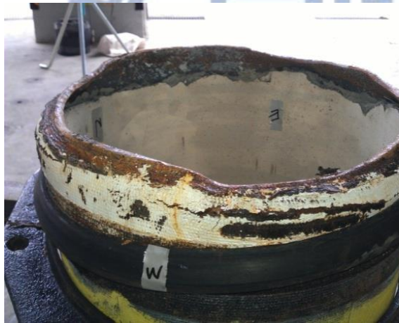
(a) 承口端鑄鐵彎曲變形內襯脫 落
