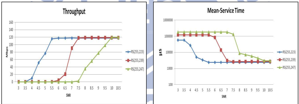
Fig. 26 Performance comparison under different RS-codec with AH-FCCMP scheme
