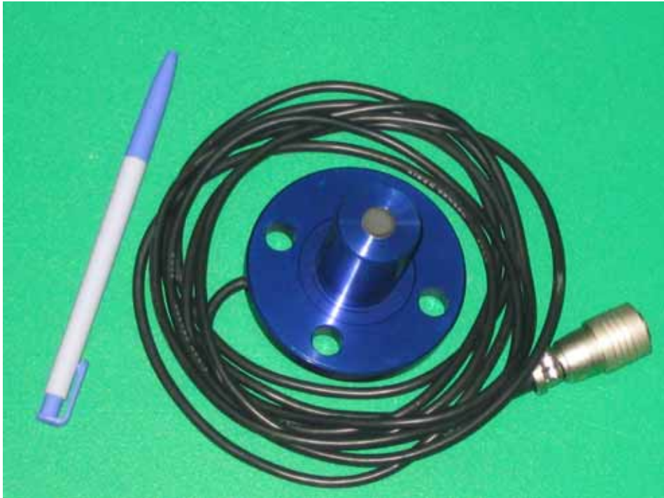
Fig. 3.3. Soil pressure transducer (Kyowa PGM-0.2KG)
