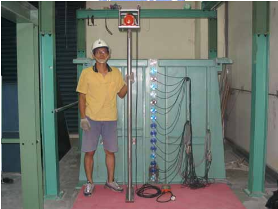
(b) Strip compactor and model wall (Side-view)
