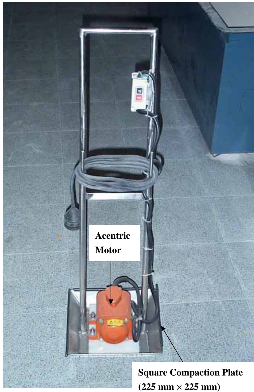
Fig. 3.7. Square vibratory soil compactor
