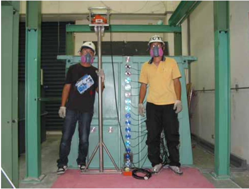
(a) Strip compactor and model wall (Front-view)
