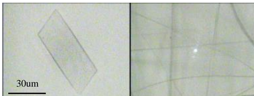
Fig. 3.1 Anhydrous and monohydrate crystal forms of L-Phe. (Left; anhydrous (plate-like), Right; monohydrate (needle-like))
