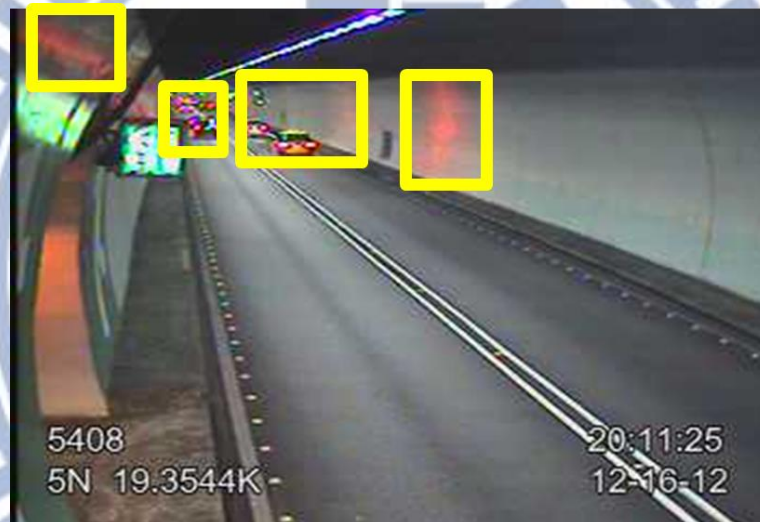
Figure 3-4. Detection fails using Mixture of Gaussians (MoG) background subtraction. Reflections on walls are treated as detected objects.
