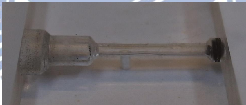
Figure 2-16. The illustration of the acrylic fixture for micropore sieve device.
