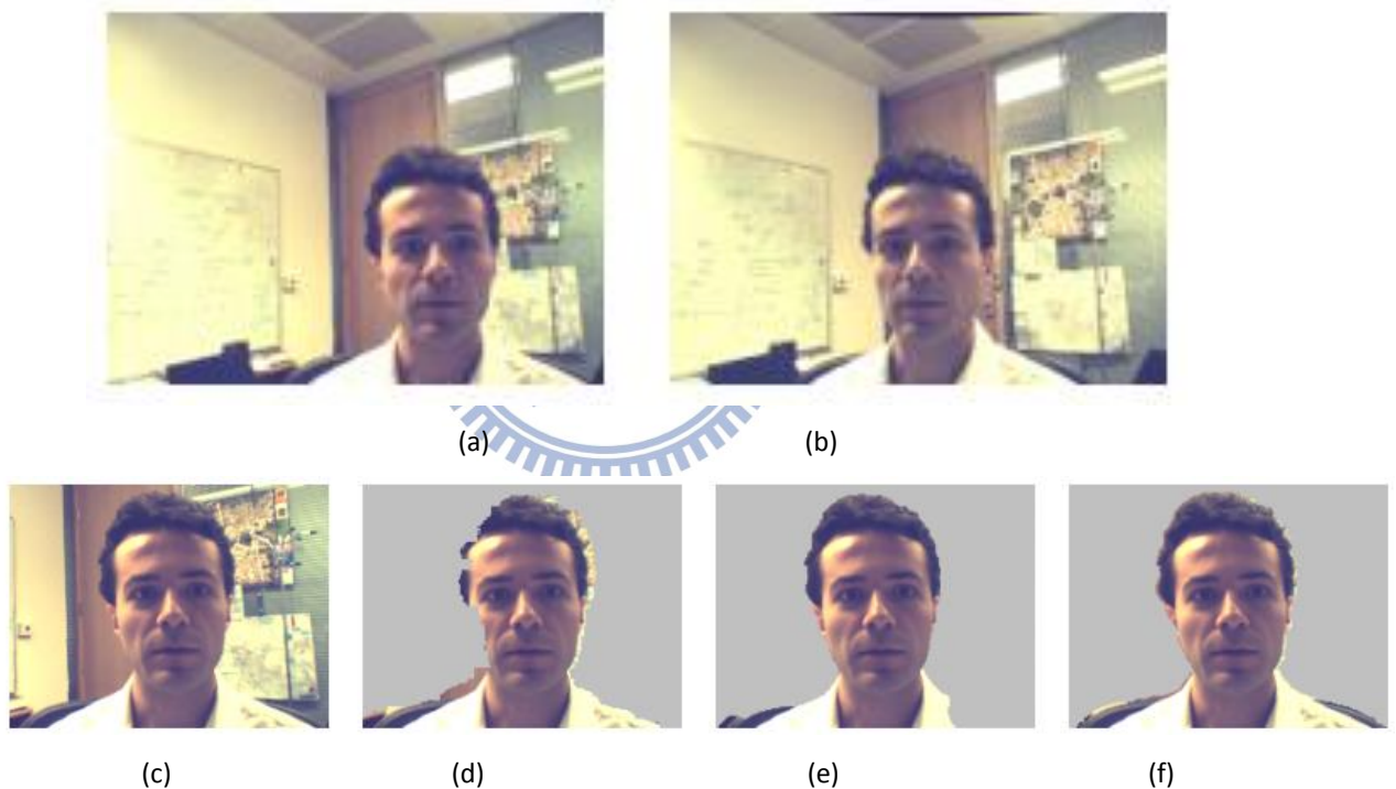
Figure 2-5 Segmentation by stereo-pairs. (a) input left view (b) input right view (c) data(left image) (d) Segmentation based on stereo (e) segmentation based on color (f) The method fuses color, contrast and stereo to achieve a more accurate segmentation.
