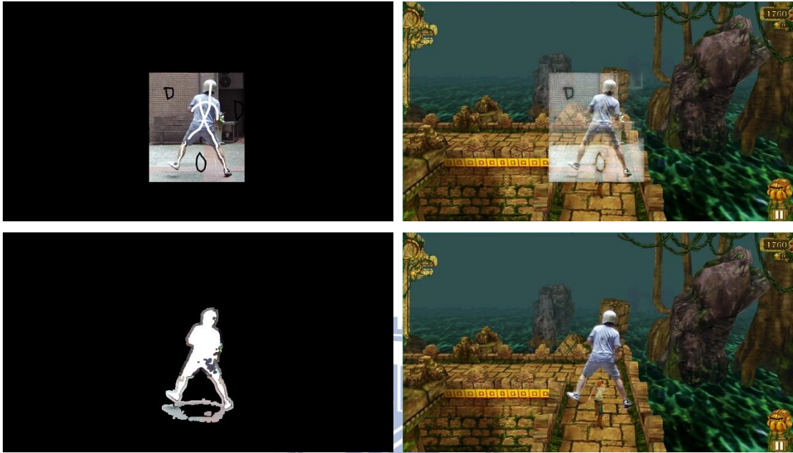
Figure4-2 Comparison between the supervised image matting method and the proposed automatic method (a) Manually selected scribbles. (b) Synthesized image based on (a) and the original ML method. (c) Automatically generated tri-map. (d) Synthesized image based on (c) and the modified ML method.
