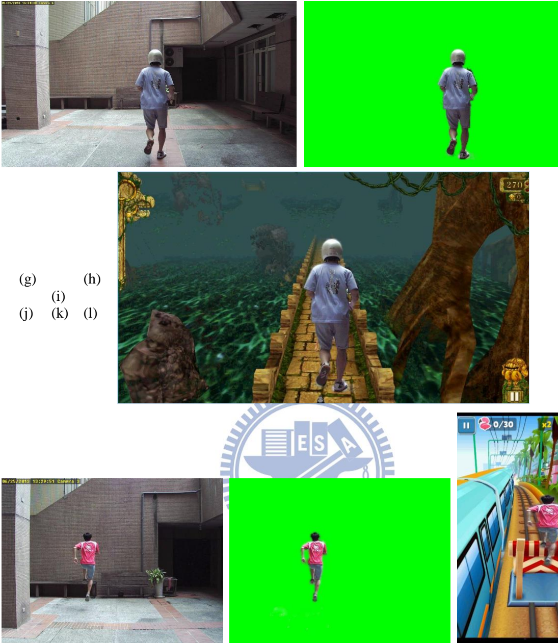
Figure 4-7 More result of the foreground object into the virtual scene. (a)(d)(g)(j) Input image. (b)(e)(h)(k) Foreground extraction. (c)(f)(i)(l) Synthesized image.
