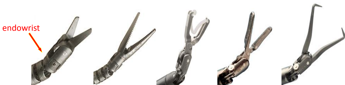
Fig. 1.11 Robotized surgical instruments of Da Vinci system[27].
