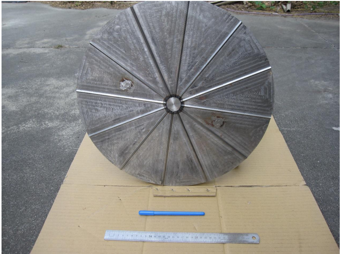
Fig. 3.5. Bottom of shearing disc with radial fins
