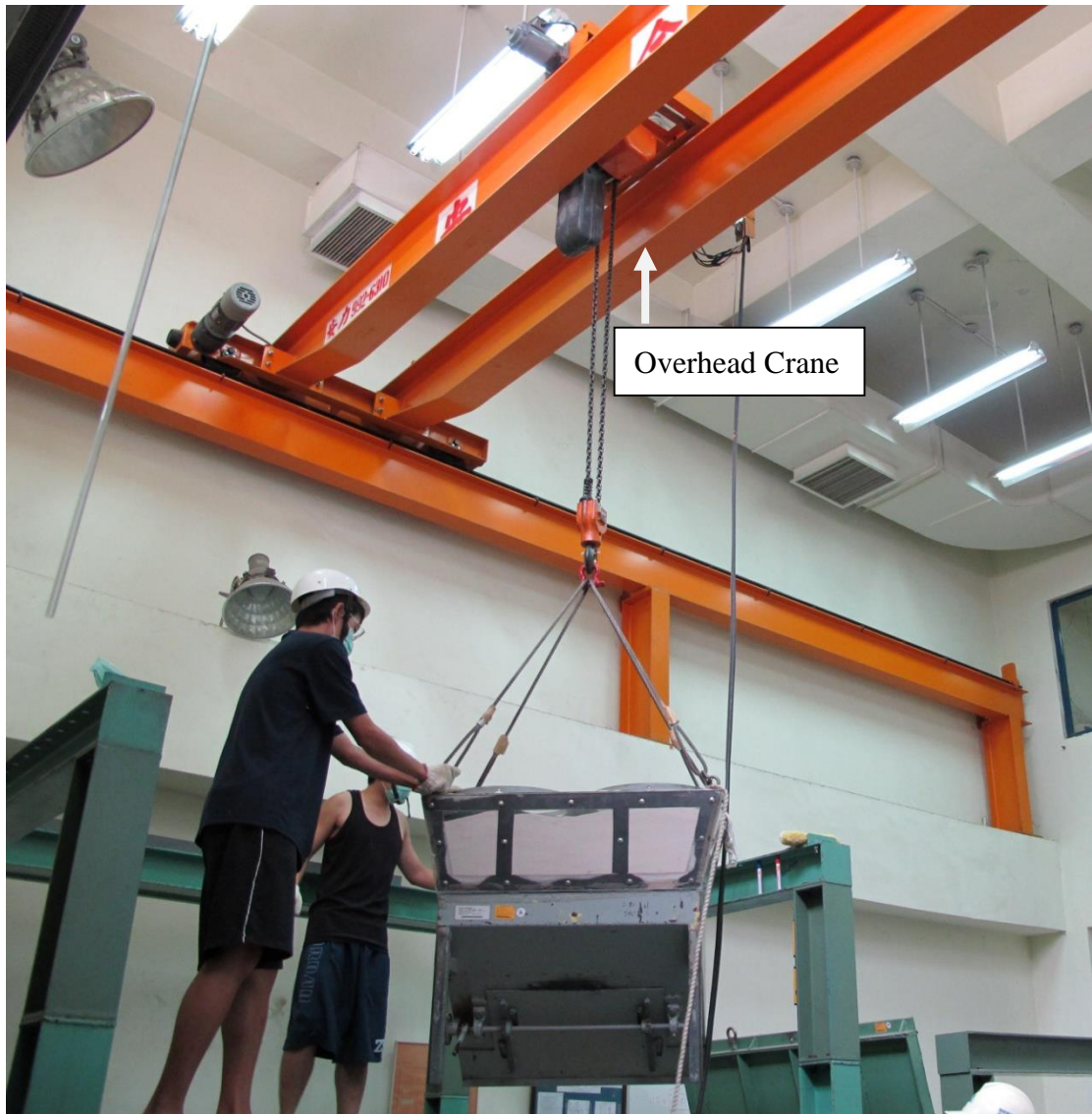
Fig. 5.3. Sand hopper lifted by overhead crane (after Chen, 2011)
