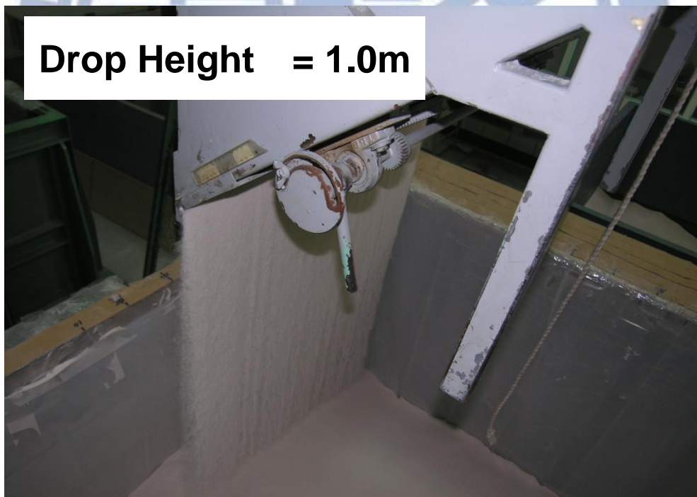
Fig. 4.5 Pluviation of Ottawa sand into soil bin (after Chen, 2011)
