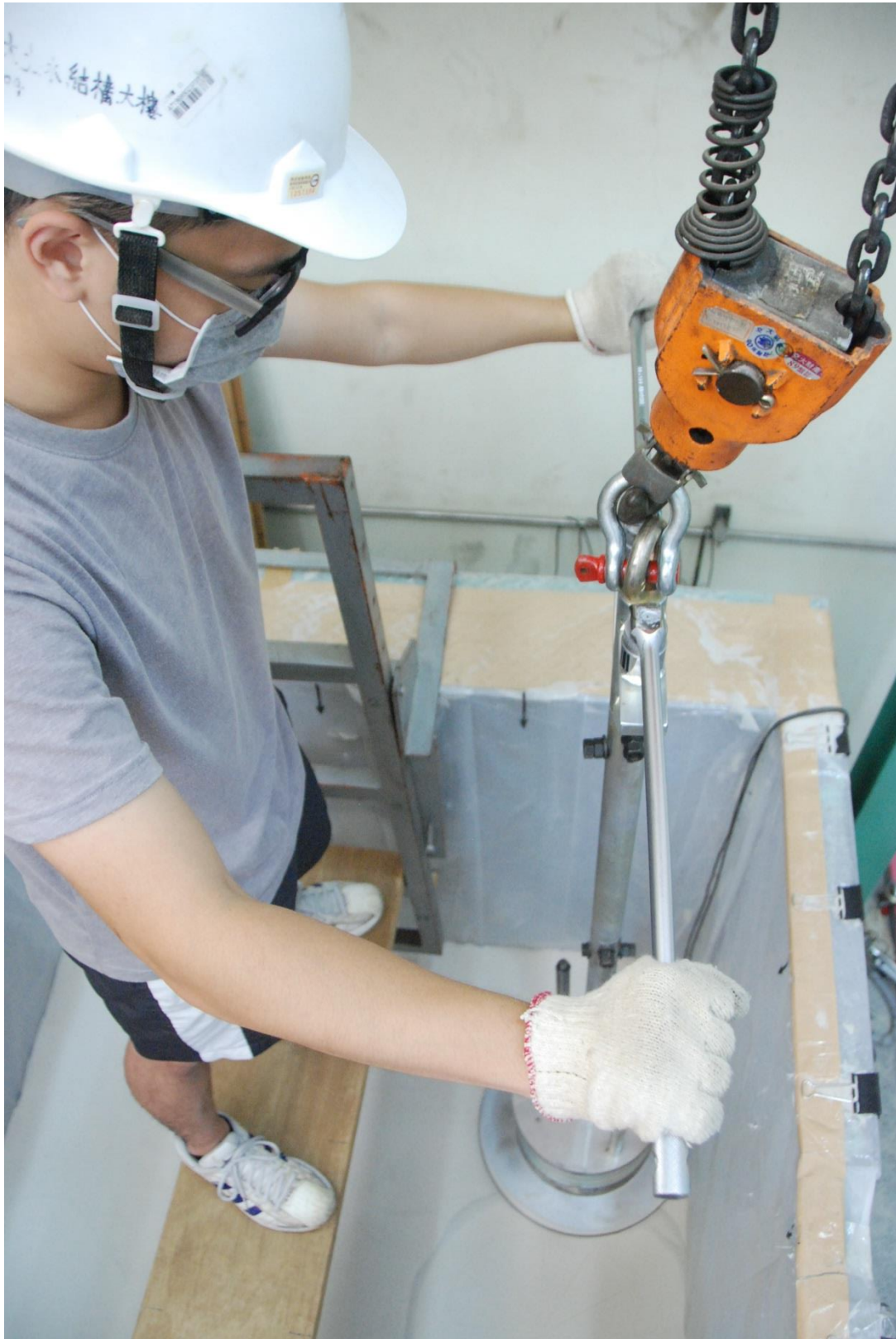
Fig. 5.17. The application of cyclic torsional shear to loose sand
