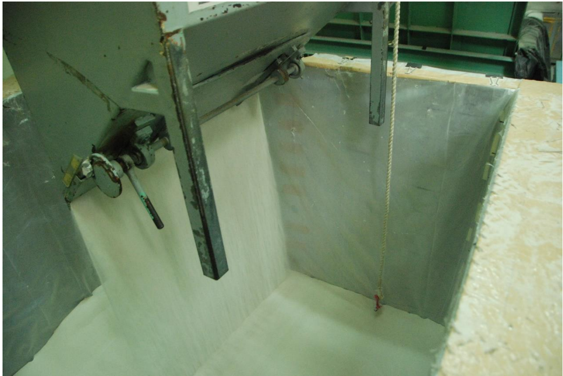
Fig. 5.4. Air-pluviation of Ottawa sand into soil bin
