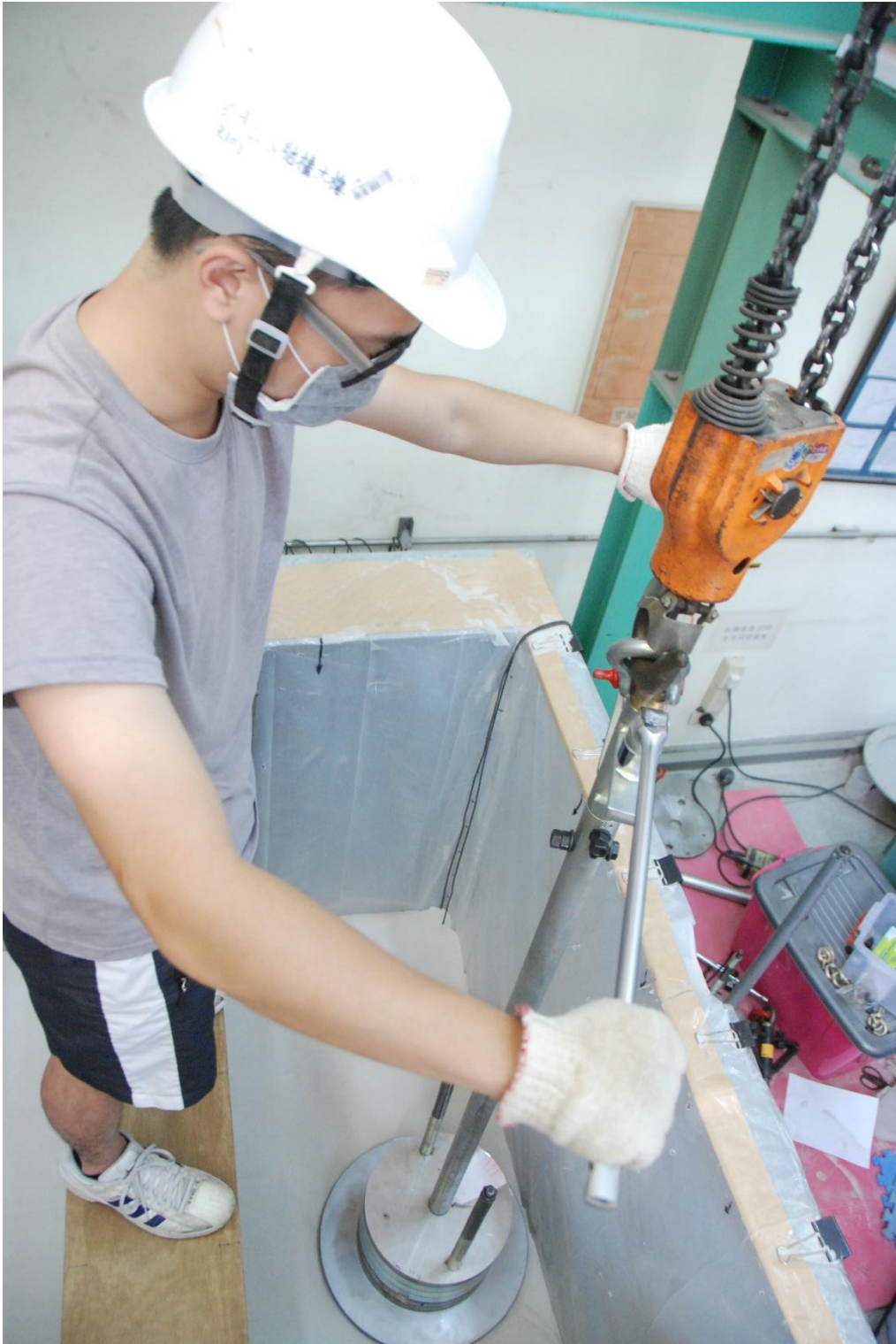
Fig. 5.11. Apply vertical static load on loose sand
