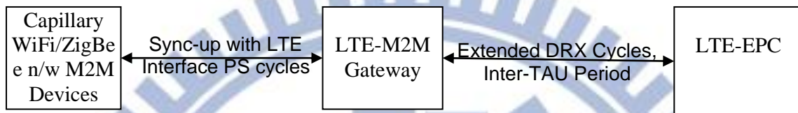
Figure 8 Power Saving Design for M2M devices
