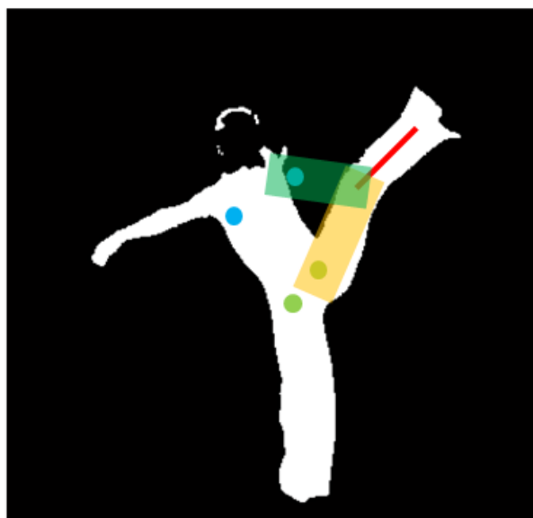
Figure 3-36 Illustration of compensation on variance from estimation of shoulder joints by cover rate.
