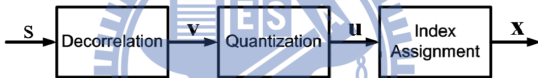
Figure 2.2: Three basic steps of source encoding procedure
