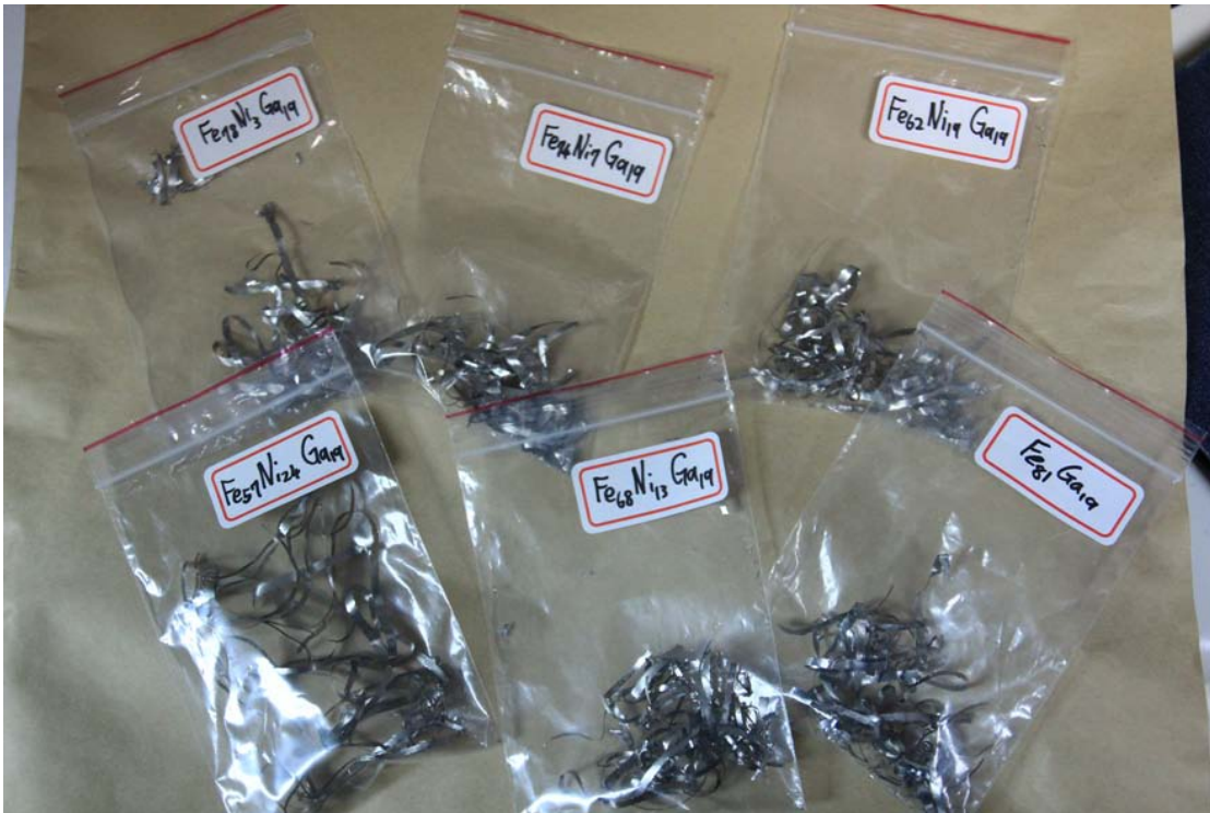
Fig. 3.4 The samples of ribbon are made by the rapid quenching melt-spun method.
