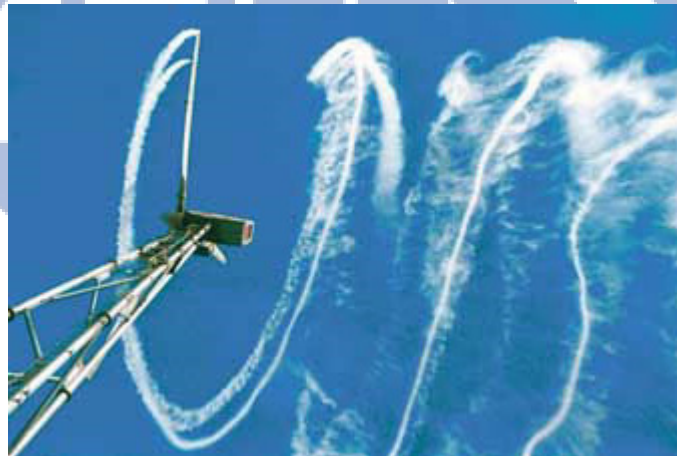
Fig. 1.4 Wake effect from wind turbine picture (Riso National Laboratory, Denmark) [22]
