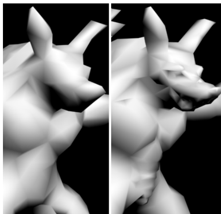
Figure 4.17: Closer comparisons between the unrefined (left) and refined (right) simplifications with 1000 faces of Armadillo.
