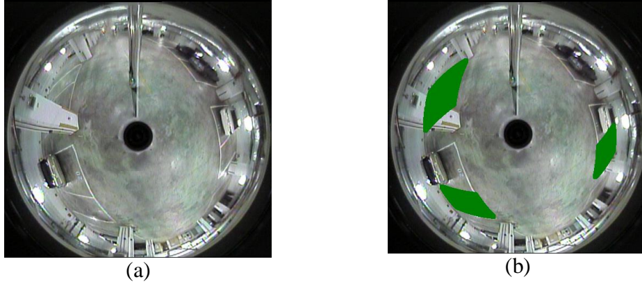
Fig. 7.14 Parking space vacancy detection. (a) Input image. (b) Vacant parking spaces marked as green regions.
