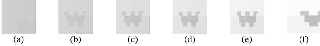
Figure 5.4. Modulated character-fragments resulting from uses of different contrast threshold values of \delta for the difference between the two representative values r_1 and r_2 . (a) \delta=0 . (b) \delta=10 . (c) \delta=20 . (d) \delta=30 . (e) \delta=40 . (f) \delta=50 .
