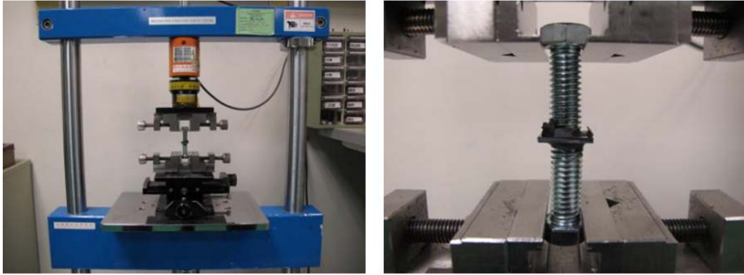
Figure 2-11 Setup before the Tensile Test and Samples after the Curing in the Tester before the Tensile Test
