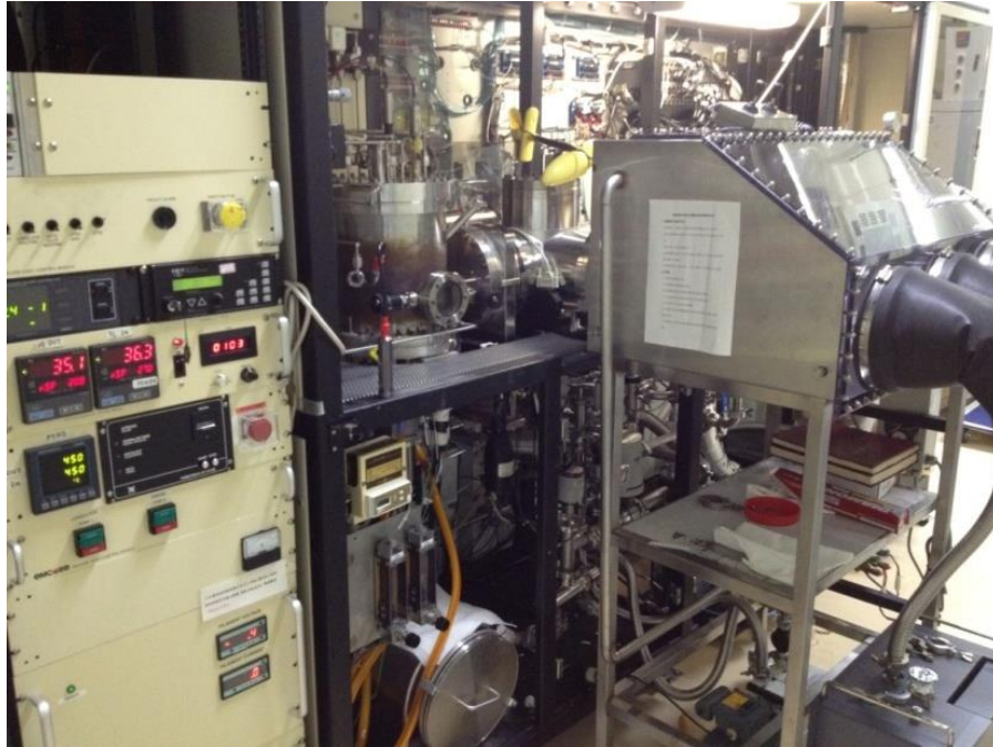
Fig. 3-1 The MOCVD EMCORE D180 system in Compound Semiconductor Devices laboratory.
