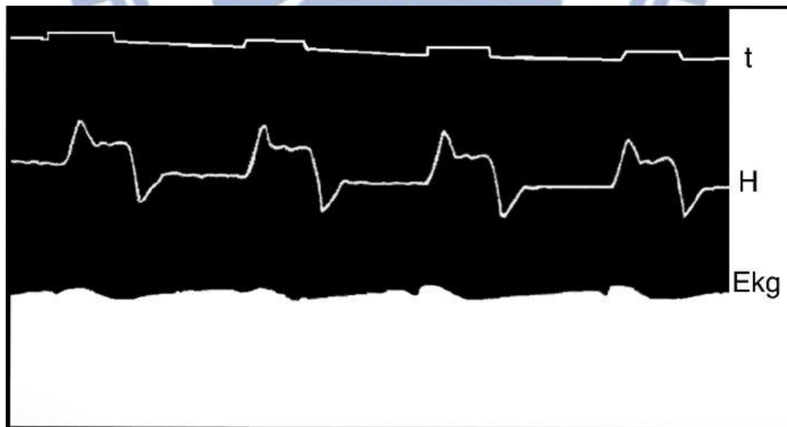
Fig. 2.2 The first human electrocardiogram recorded by Waller in 1887. t=time in seconds, Ekg=electrocardiogram, h=chest wall movement. [37]
