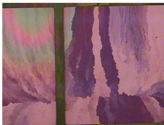
Fig. 5. Polarized optical microscopy of BC TES-ADT OTFT with Ni electrode (Mag. X200).
