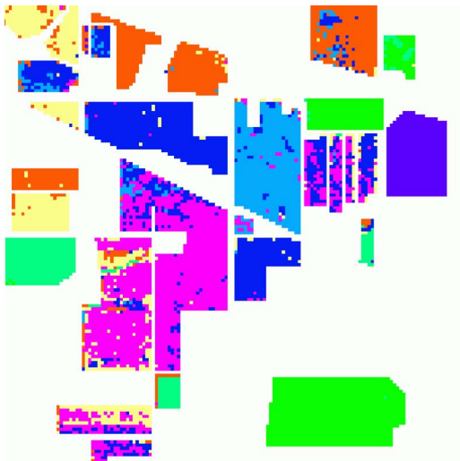
Fig. 6. Thematic map resulting from the classification of the area of Fig. 1 by NWEF with ML classifier ( N_i = 300, p = 14 ).
