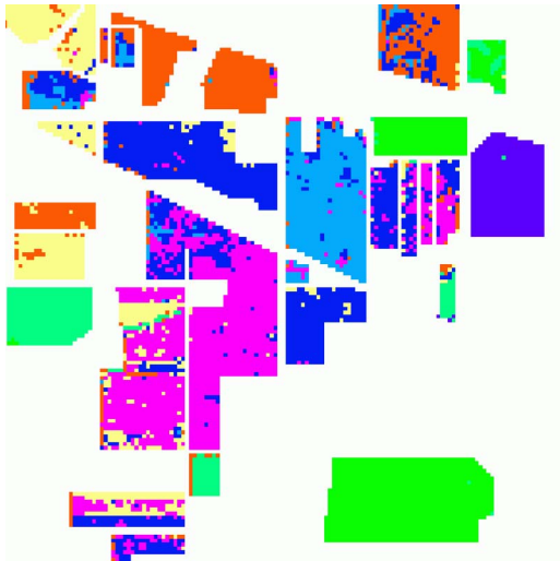
Fig. 5. Thematic map resulting from the classification of the area of Fig. 1 by ICA with ML classifier ( N_i = 300, p = 9 ).
