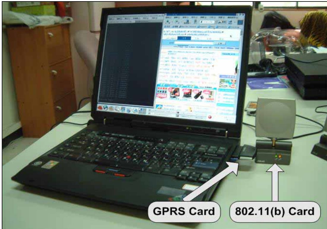
Figure 5.1-3: Each notebook computer is equipped with an IEEE 802.11(b) WLAN interface card and a GPRS interface card.
